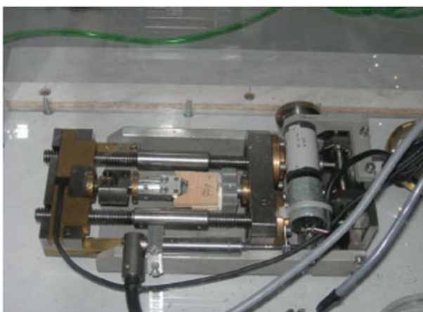
Figure 1 Loading wedge-splitting stage inside the climate Plexiglass box.
