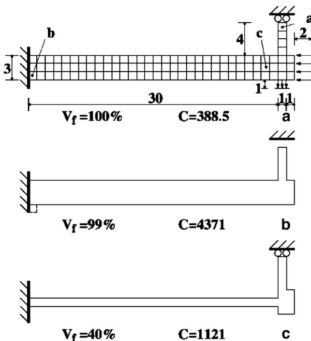
**Fig. 4** The example in a brief note by Zhou and Rozvany (2001). **a** Problem statement, **b** highly non-optimal solution for a volume fraction of 99% by the ESO method, **c** intuitively “good” design for a volume fraction of 40%
