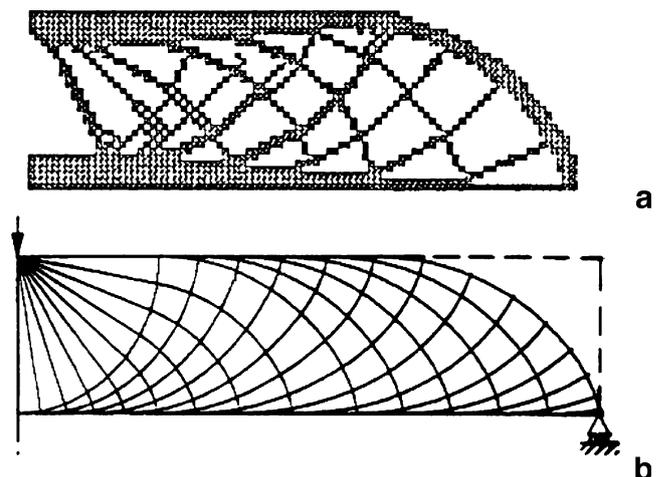
**Fig. 2** **a** A very early SIMP solution for the “MBB beam”, presented in 1990 (Rozvany and Zhou 1991). **b** The corresponding exact analytical truss solution (Lewinski et al. 1994)
