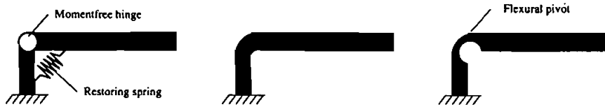
Fig. 1. A rigid body mechanism (left), a distributed compliant mechanism (center), and a lumped compliant mechanism (right).
