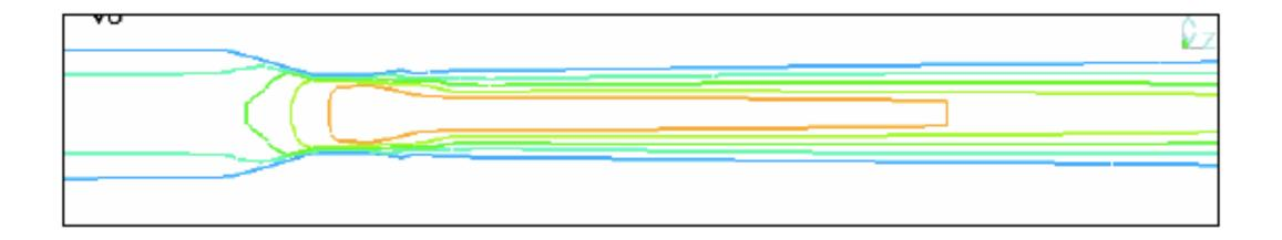
Fluid flow in sudden axisymmetric constriction
