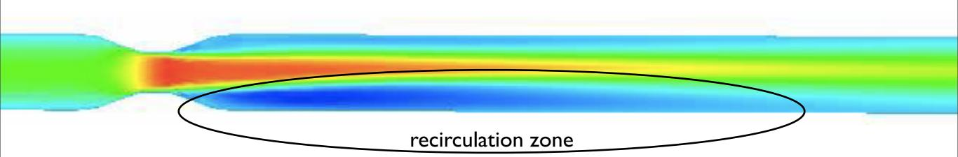
Fluid flow in sudden axisymmetric constriction
