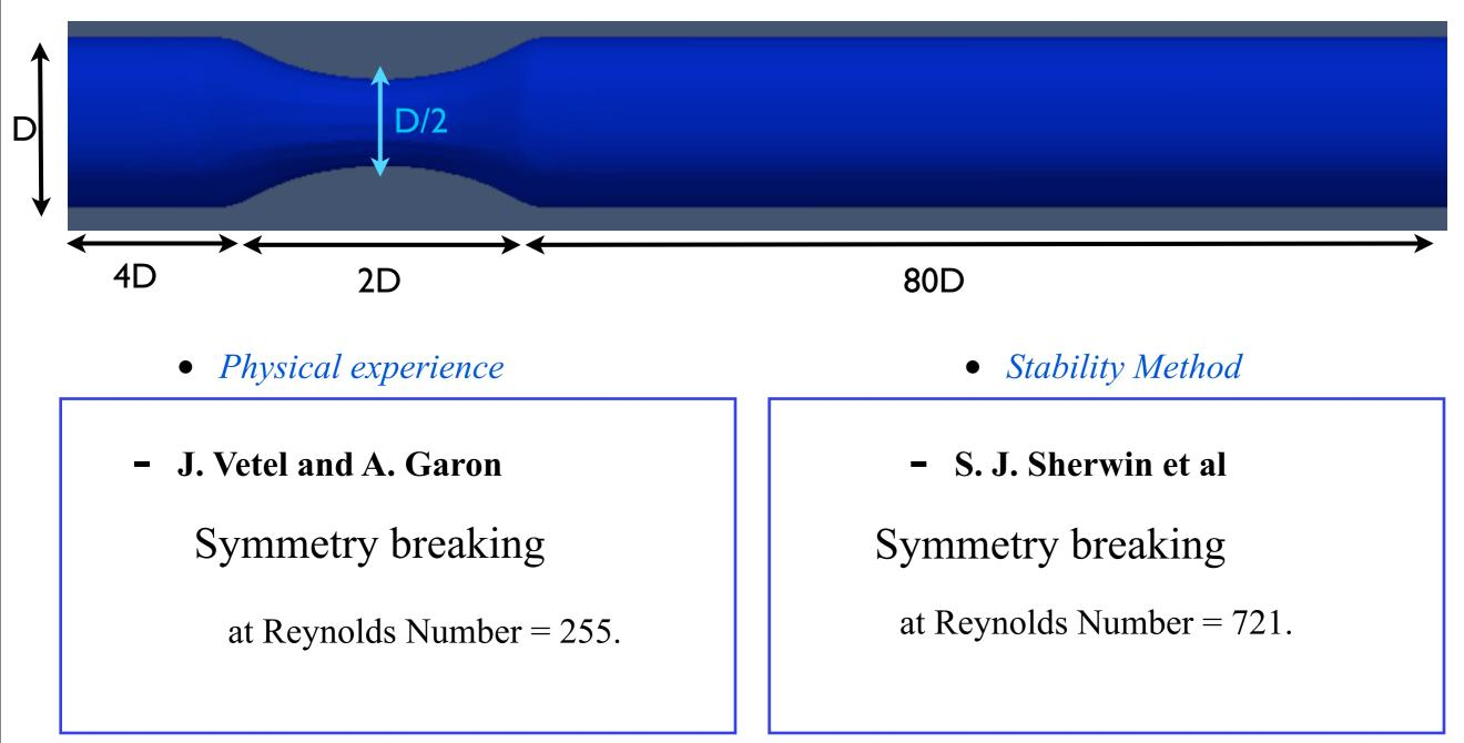
Fluid flow in a sudden axisymmetric constriction
